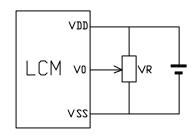
$V_{DD\sim}V_0$ : LCD Driving voltage
